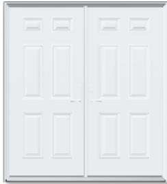
Two doors side by side, both of which are hinged and operable. The first door to open is active, the second passive. The doors are separated by an astragal mounted to the passive panel, and may only be hinged on the jambs.
